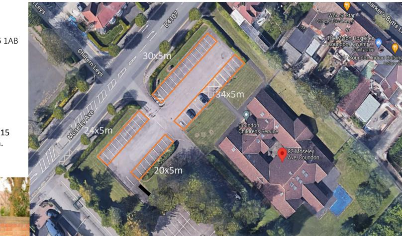
This car park is closed during the night time. The proposal is to install 42 x 7 kW charging bollards and make them accessible to the nearby residents (up to 10mins walking distance) who do not have off street parking facility. Battery will allow for a smaller grid connection.
